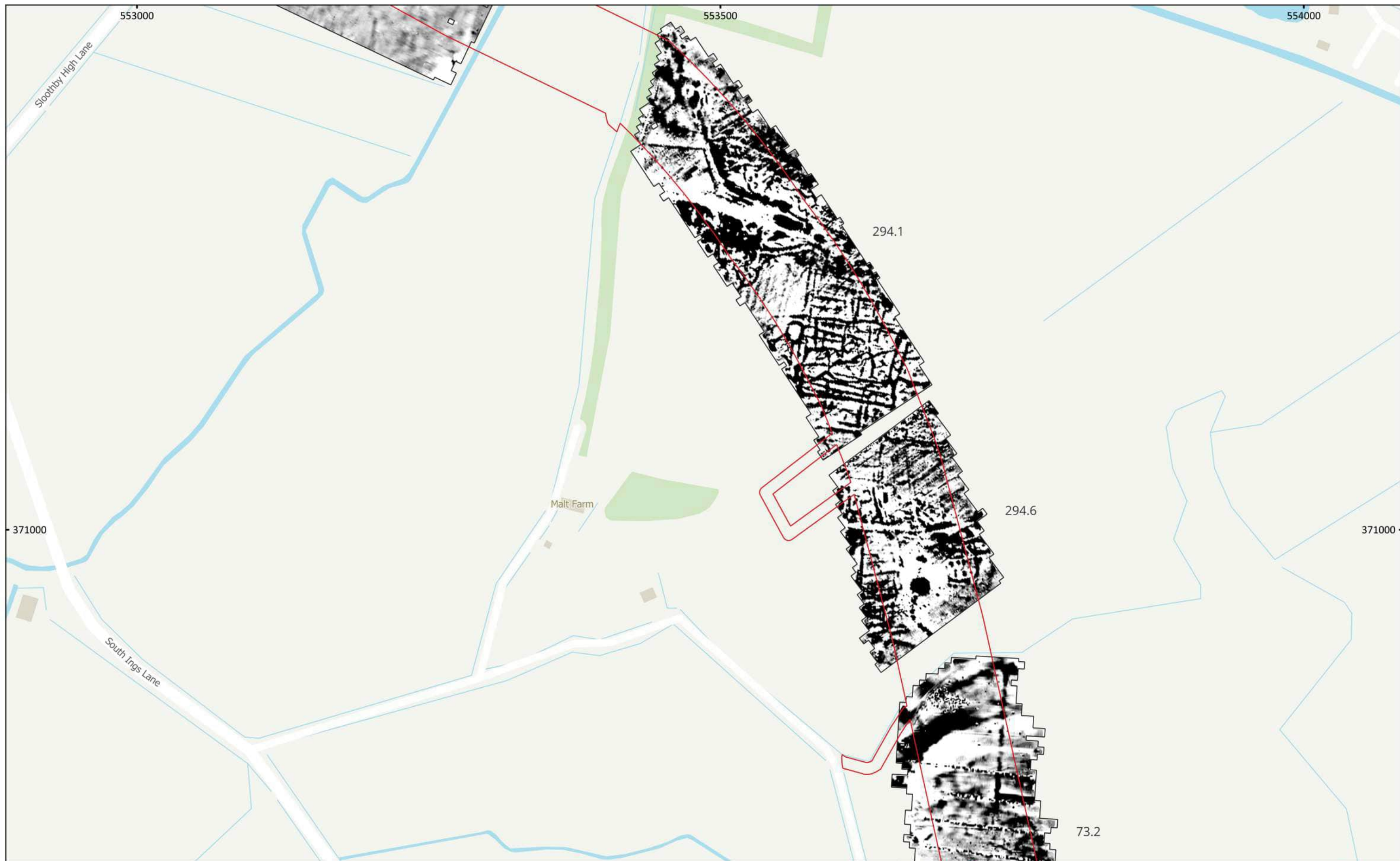
MSTF1592: ODOW - Onshore Archaeological Geophysics Figure 47 - Magnetic Total Field (Lower Sensor) (Overview) (Area ECC2) 1:3,000 @ A3 Copyright Magnitude Surveys Ltd 2024 Contains Ordnance Survey data © Crown Copyright and database right 2024
