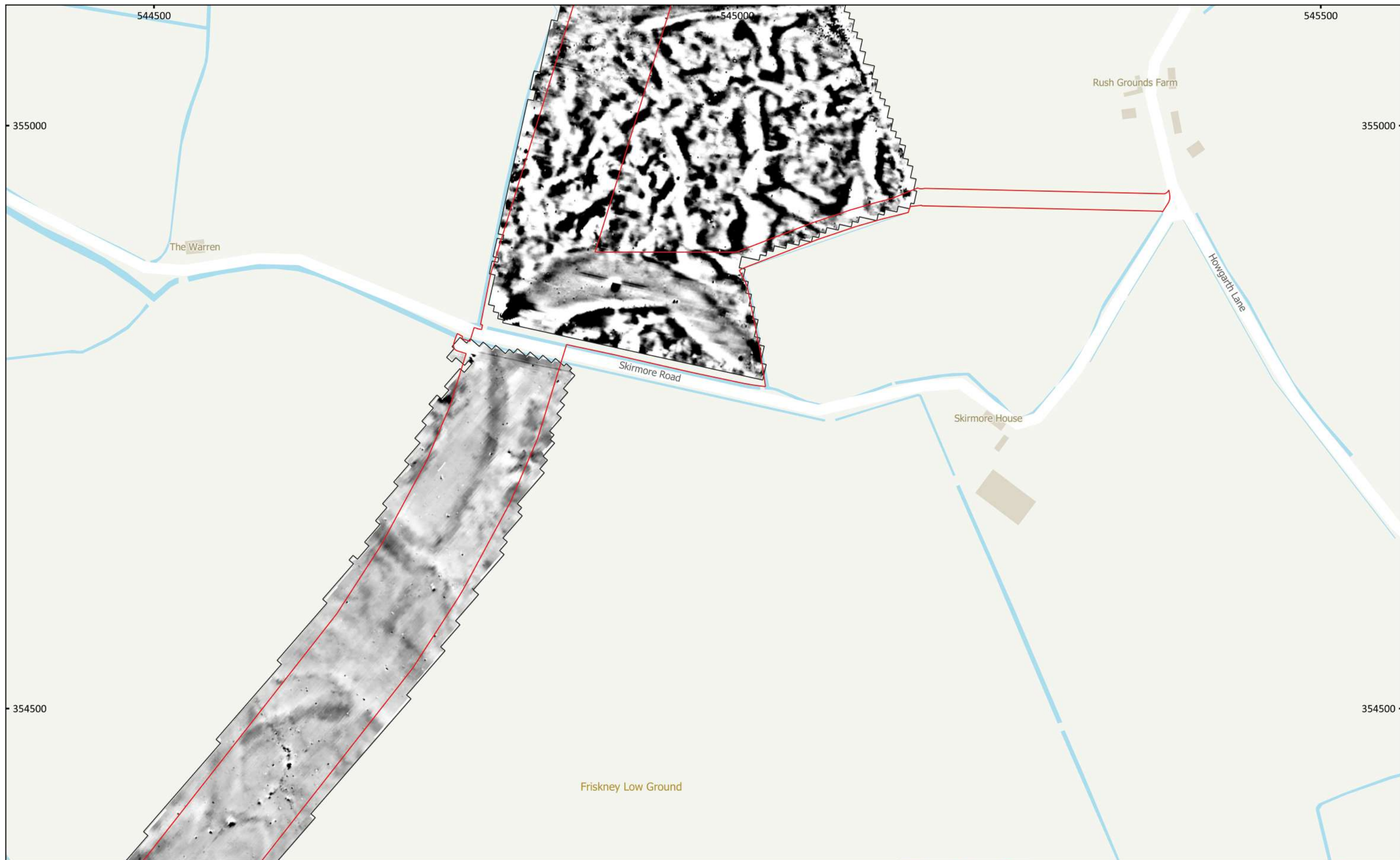
MSTF1592: ODOW - Onshore Archaeological Geophysics Figure 173 - Magnetic Total Field (Lower Sensor) (Overview) (Area ECC7) 1:3,000 @ A3 Copyright Magnitude Surveys Ltd 2024 Contains Ordnance Survey data © Crown Copyright and database right 2024
