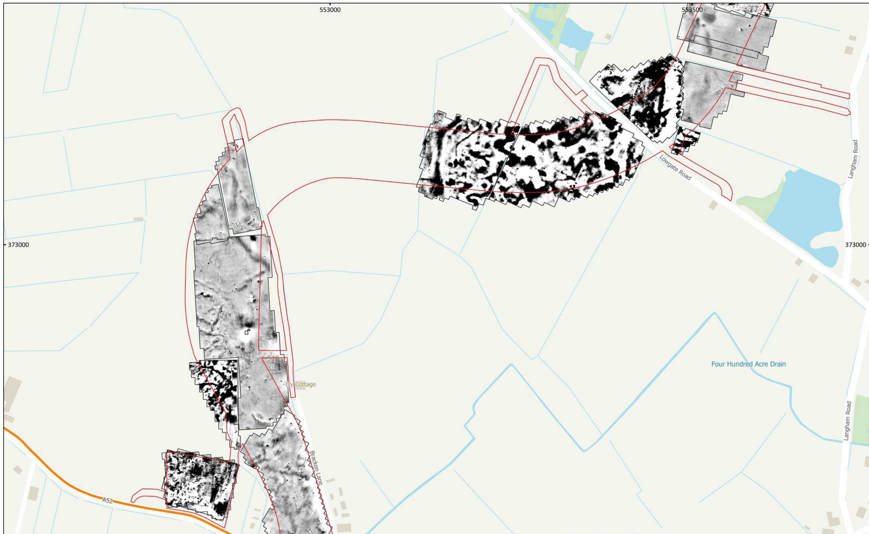
MSTF1592: ODOV - Onshore Archaeological Geophysics Figure 33 - Magnetic Total Field (Lower Sensor) (Overview) (Area ECC1) 1:3,000 @ A3 Copyright Magnitude Surveys Ltd 2024 Contains Ordnance Survey data © Crown Copyright and database right 2024
